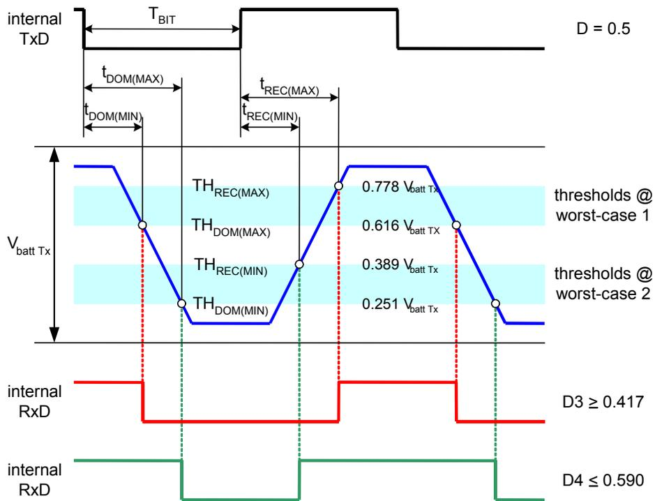
FIGURE E1—RELATION BETWEEN PROPAGATION DELAY AND DUTY CYCLE
