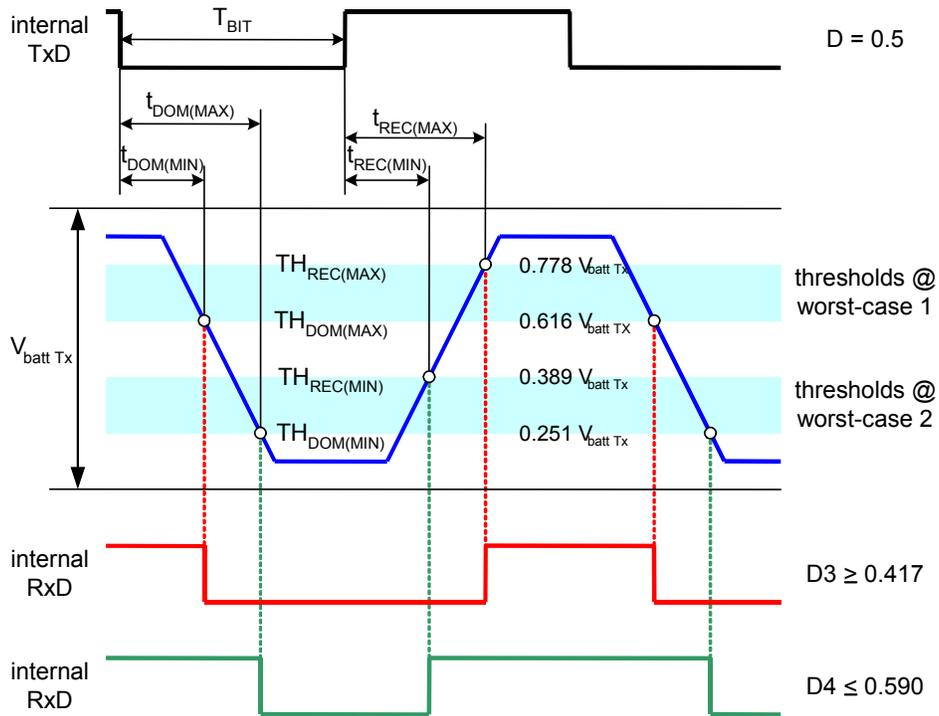
FIGURE C1—RELATION BETWEEN PROPAGATION DELAY AND DUTY CYCLE
