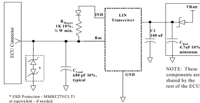
FIGURE 4—TYPICAL LIN MASTER BUS INTERFACE
