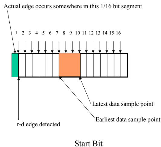
FIGURE 2—BIT SAMPLE TIMING
